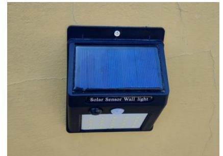
Tigergarh Wildlife Resort's solar sensor lights turn off automatically during daytime and at night light up only when there is someone within a radius of twelve feet.
