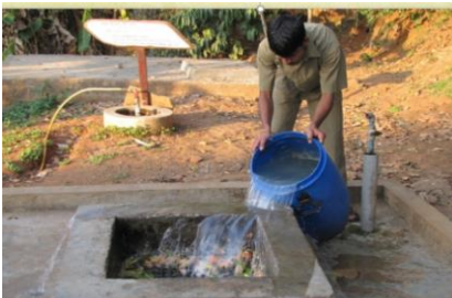
A biogas unit at Evolve Back Kabini utilises methane produced from kitchen waste for cooking.
